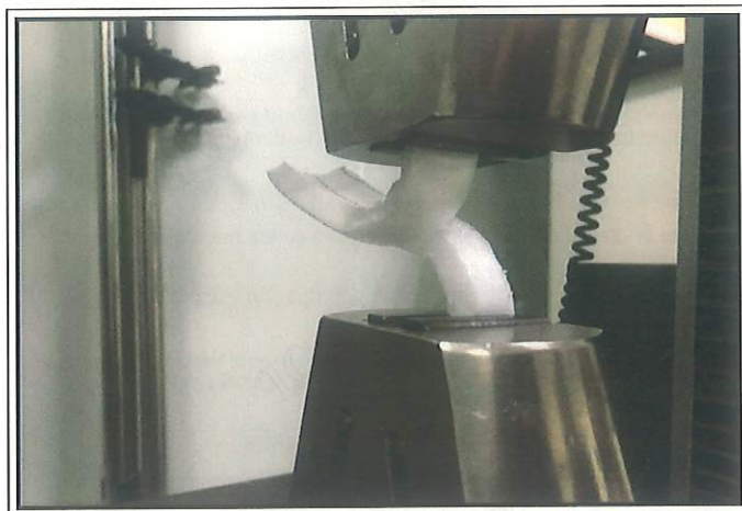
During tear strength test
