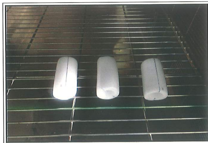
During dimensional stability test
